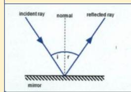
Light travels in straight lines. It reflects off mirrors according to the law of reflection which states that the angle of incidence (i) = angle of reflection (r).
